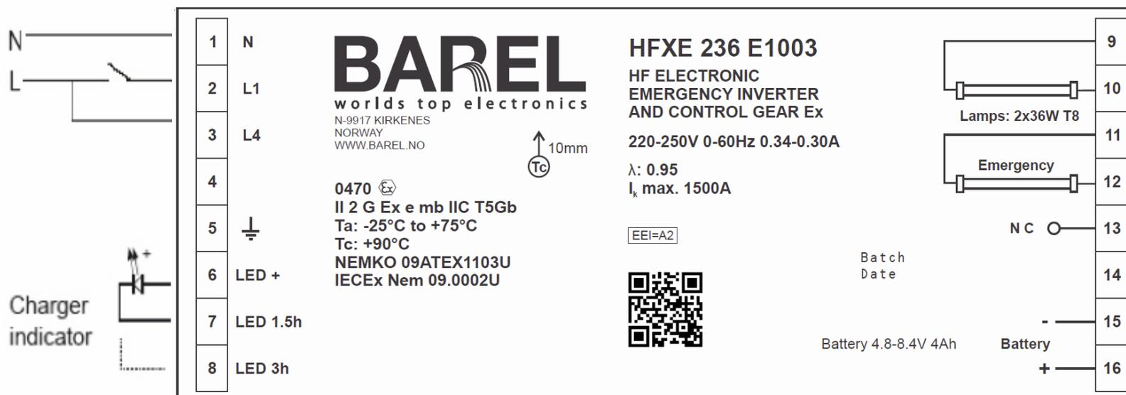
Connector 13 “NC” has no internal connection, and may be used for battery-cable extension.
